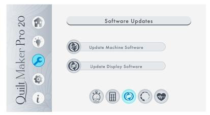
After downloading the updated software to a USB drive, insert the drive in the designated USB port on the bottom of the front display. Look for the message in the bottom bar that confirms a USB drive has been inserted. If it doesn't appear, reinsert the USB drive. Then touch the **Update** button. Press the **Home** button to return to the Main screen.
