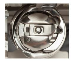
**NOTE**: Do not insert the bobbin case into the machine by lifting the lever on bobbin case. Use the lever only for removing the bobbin case.
