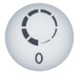
The Easy-Set Tension<sup>™</sup> shows the top tension setting as a numeric value on the display. The number on the button indicates the current tension, which is set by manually turning the tension knob. After you establish the tension setting for a particular thread (brand, weight, and color), record the value so you can easily return to that tension setting when using that specific thread again.
