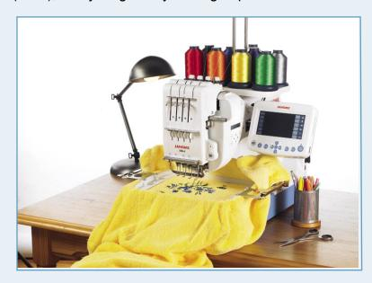
RCS (Remote Computer Screen) LCD colour touch screen. Large viewing area. USB and ATA PC Card slots on side. Attaches to MB-4 or is free standing.
