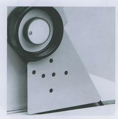
Belt guard on the handwheel
